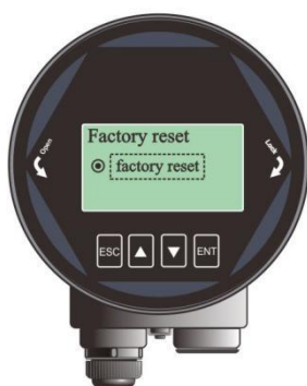
Figure 6-14. Factory reset interface
