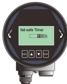
Figure 6-23. Fail-safe timer interface
