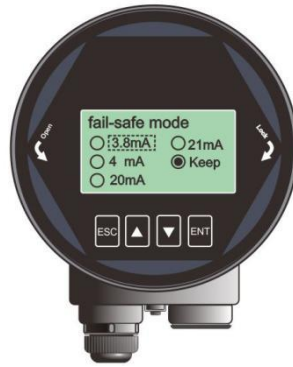
Figure 6-22. Fail-safe mode interface
