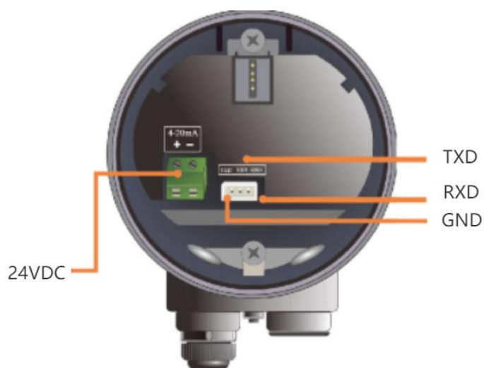
Figure 5-2. 2-wire product wiring diagram
