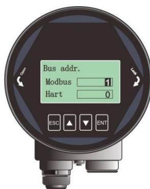
Figure 6-20. Bus address interface
