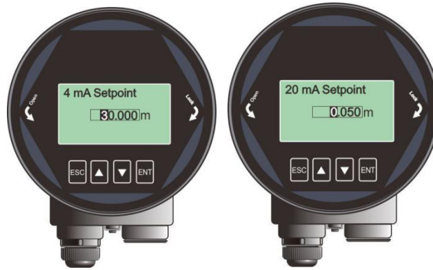
Figure 6-17. 4mA/20mA setpoint interface
